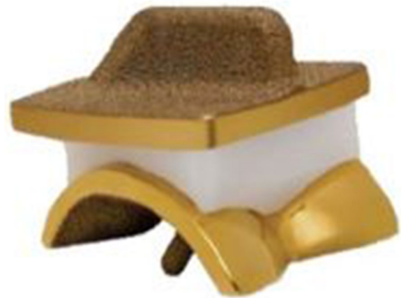
Fig. 1 The CCI Evolution TAR implant (Van Straten Medical). The three components from top to bottom: tibial CoCrMo component, polyethylene liner, talar CoCrMo component
