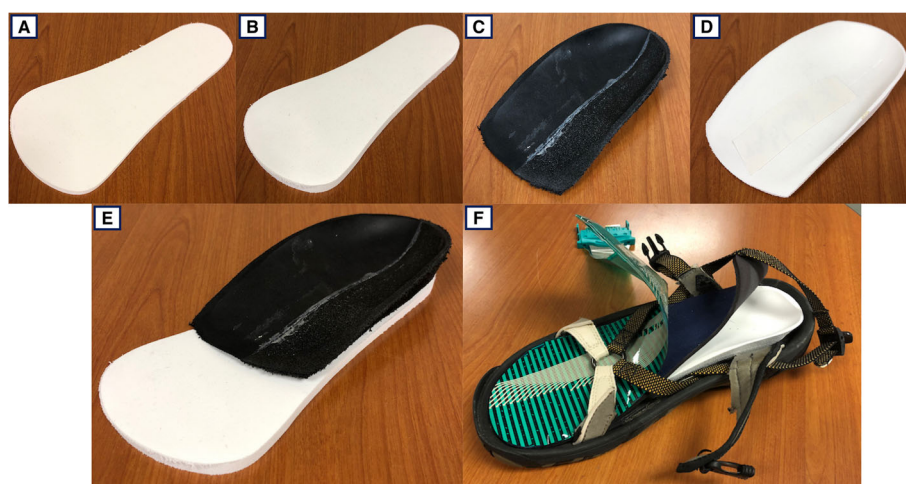
Fig. 1 Insoles and standardized sandal set-up used for walking trials. A 3 mm flat control (FLAT). B 5° lateral wedge (WEDG). C Variable-stiffness arch support (V-ARCH). D Uniform-stiffness arch support (U-ARCH). E Example of supported lateral wedge (WEDG+V-ARCH shown). F Sandal setup with insole, neoprene topcover, and plantar pressure sensor
