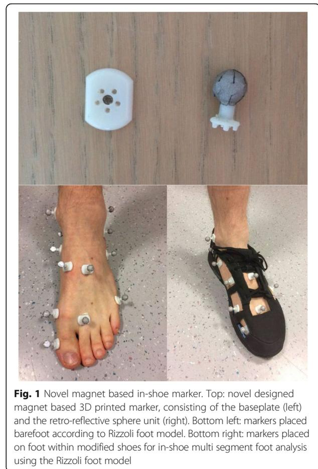
**Fig. 1** Novel magnet based in-shoe marker. Top: novel designed magnet based 3D printed marker, consisting of the baseplate (left) and the retro-reflective sphere unit (right). Bottom left: markers placed barefoot according to Rizzoli foot model. Bottom right: markers placed on foot within modified shoes for in-shoe multi segment foot analysis using the Rizzoli foot model
