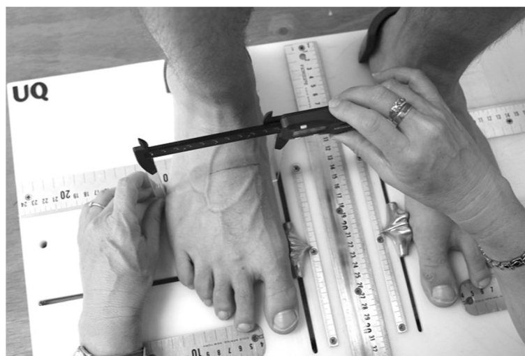
Fig. 8 Midfoot width measured in weight bearing
