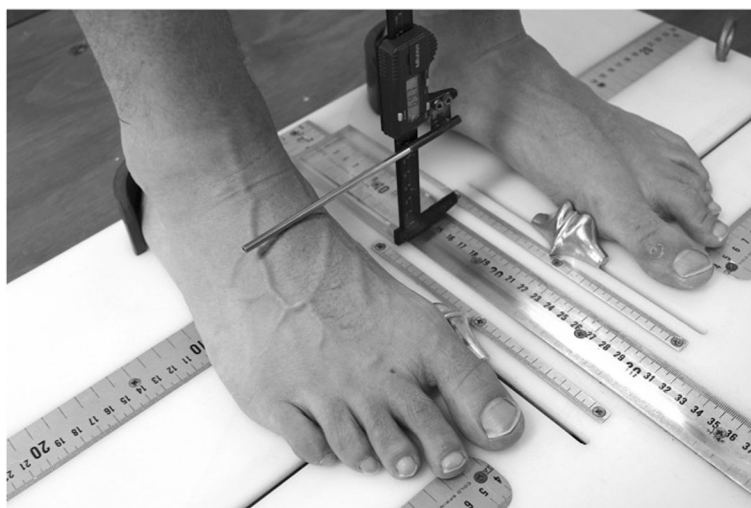
Fig. 10 Midfoot arch height measurement
