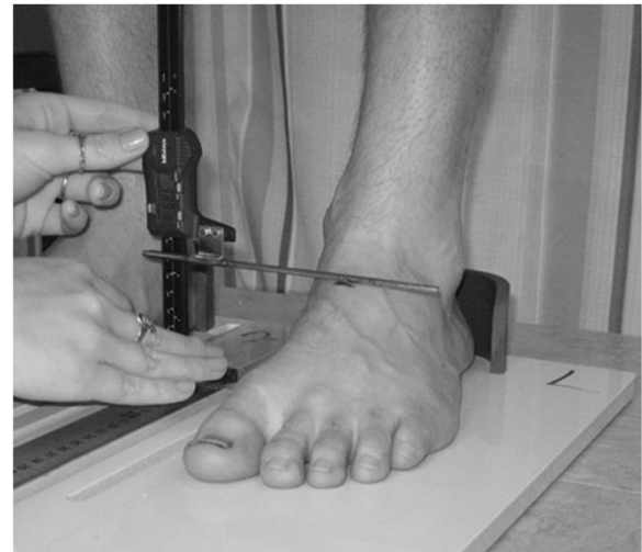
Figure 3 Measurement device for dorsal arch height using a modified digital caliper (Model #700-126, Mitutoyo America Corp, Aurora, IL 60502). A 1.2 \times 5.0 \times 10.0 cm plastic block holds the caliper vertically. The arch height is measured by a sliding metal rod extension of the caliper arm.
