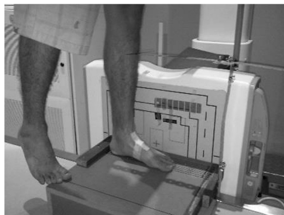
Figure 2 Platform constructed in order to standardize position of foot and leg relative to the X-ray camera and plate.
