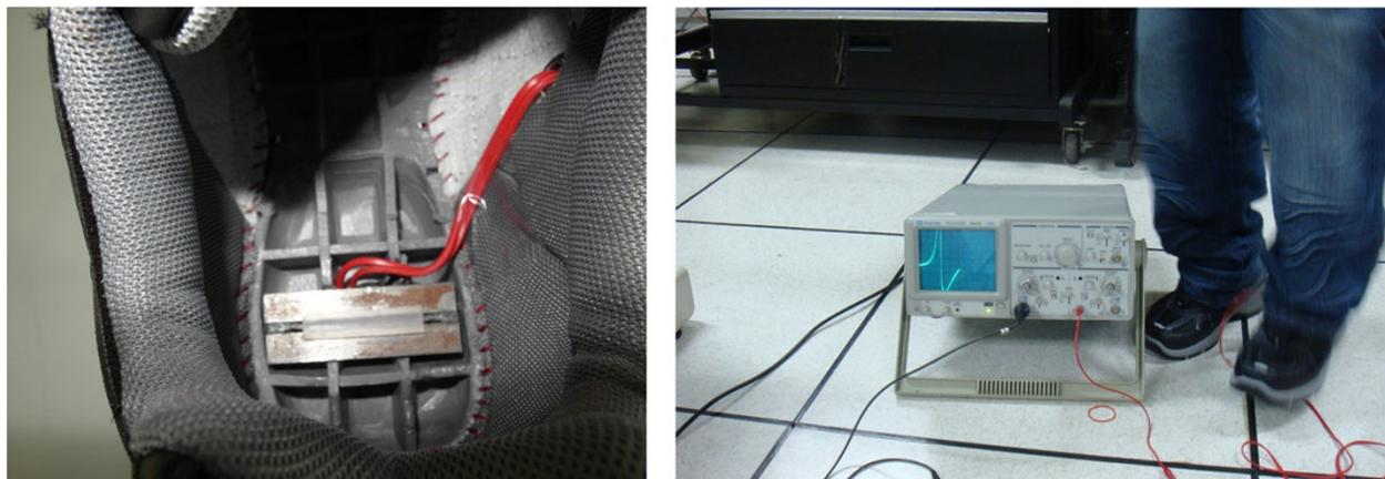
**Figure 1** Testers wore shoes for generating voltage measurements
