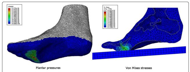
Figure 1 Example of the results of a FEM simulation with ulcerated subject's boundary conditions: Plantar pressures (left) and Von Mises internal stresses (right).
