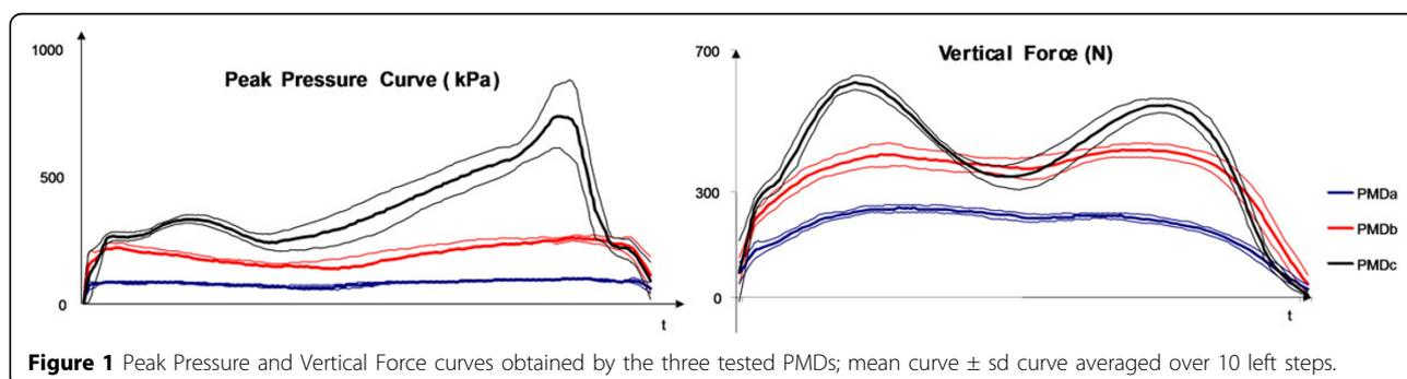
**Figure 1** Peak Pressure and Vertical Force curves obtained by the three tested PMDs; mean curve  $\pm$  sd curve averaged over 10 left steps.
