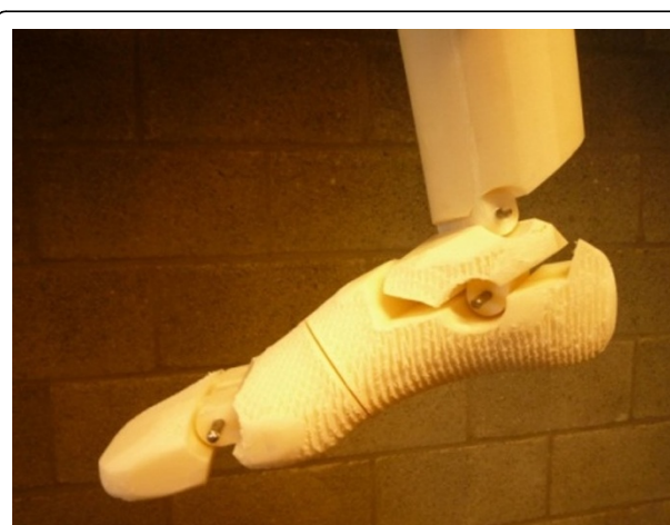
Figure 1 Initial design of the artificial foot
