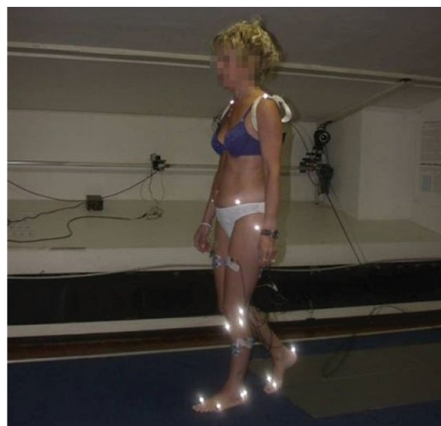
Figure 1 A BOX Ankle patient instrumented with the marker-set of the protocol utilised.
