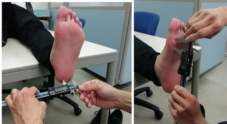
Fig. 2 Evaluation of TPDS using a digital caliper. A digital caliper was used to measure TPDS of both soles of the participants' feet. To measure TPDS, the participants closed their eyes, the soles of their feet were then brought into contact with the two points of the digital caliper, and the minimum distance between the two points of the calipers at which the participants could identify the two points distinctly was measured. TPDS: two-point discrimination sense
