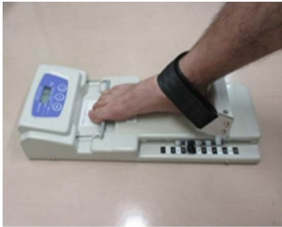
Fig. 1 Evaluation of TGF using a toe muscle strength measuring device. To measure TGF, the participants sat in a chair barefoot. The participants then pulled a bar attached to the device using their toes, while their ankle and the sole of their foot were fixed to the device using a belt on the floor. We paid attention to the participants' motion to ensure that their ankle and the sole of their foot were attached to the device and to prevent other compensatory movements while measuring the TGF. TGF: toe grip force
