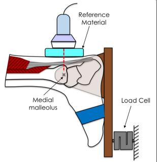
**Fig. 1** Schematic of the experimental setup. The foot was securely attached to a dynamometer with a wooden board at a fixed angle of 0° of dorsiflexion. The force measured by the load cell was proportional to the torque exerted at the ankle level. The ultrasound probe was placed in a longitudinal scan at the level of the medial malleolus
