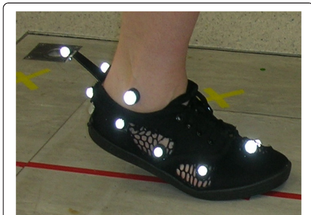
Fig. 1 Depicts the webbed upper of the modified shoe during gait analysis with the Oxford multi-segment foot model marker set in situ
