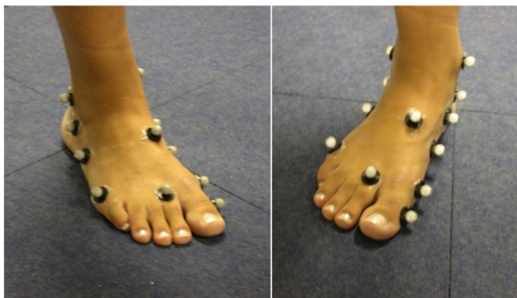
Figure 8 Marker-set for multisegment foot tracking. Marker-set for the multi-segment model of foot tracking by Leardini et al. [39]. It includes those three foot markers as in Figure 7.
