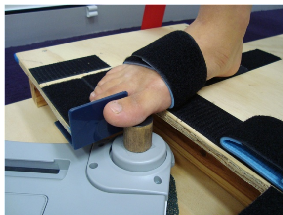
Fig. 2 Close up image of the position of the foot on the platform secured with Velcro and the position of the sensor placed under the interphalangeal joint of the big toe
