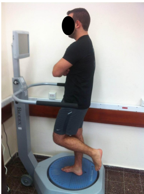
Fig. 1 Postural control testing. Note. Participants stood in single-limb stance in the central region of the Biodex Stability System platform. Participants were instructed to look straight ahead and to keep the platform as motionless as possible for 20 sec
