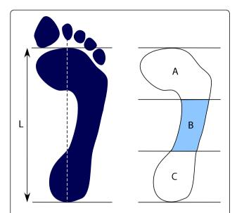
**Figure 2 Calculation of the AI.** The length of the footprint excluding the toes (L) is divided into equal thirds. The AI is then calculated as the area of the middle third of the footprint divided by the entire footprint area (AI = B/A + B + C).
