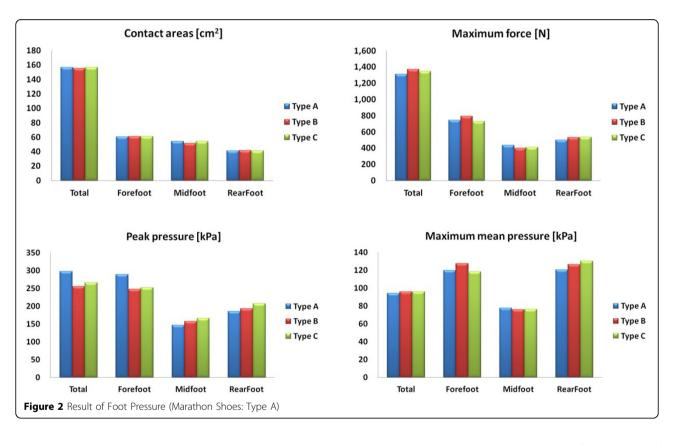
was collected by using a pressure device at a sampling rate of 100Hz. The statistical analysis was carried out by using the MINITAB R15 package, specifically One-way ANOVA ( $\alpha$ =.05). Type A shoe has the lowest peak pressure at total mask. Generally, the Type A shoe had overall lower values for the maximum force and maximum mean pressure variables compared to Type B, C shoe conditions.
